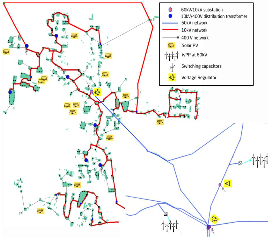
Fig. Active distribution network with a large share of weather-dependent generation
